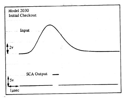
Now increase the amplifier output further until the SCA output pulse disappears. Verify the peak amplitude of the input signal to be approximately 6v.
