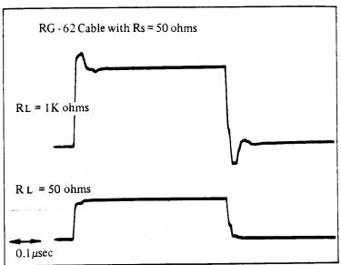
The picture below illustrates the same pulses with a source mismatch caused by driving the cables with the transistor switches directly. The waveforms indicate how important and effective source matching is in eliminating instabilities which cause phenomena such as multiple counting or triggering. For this reason the Model 2031 provides source matched outputs, and load end terminations are not necessary.
